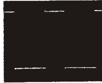
FIG. 12.9. Overshoot due to incorrectly adjusted potentiometers
