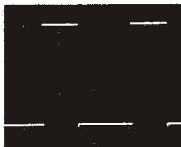
FIG. 12.7. Preset potentiometers correctly adjusted
